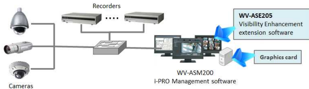
Figure 3: System configuration example of Panasonic Visibility Enhancement Software.
