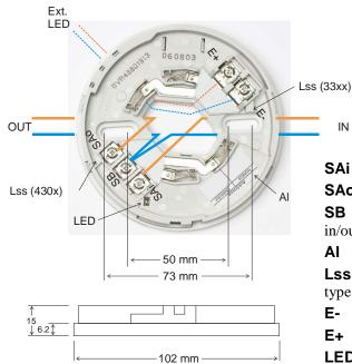
The detector plugged in the base is connected on the SAo side.
